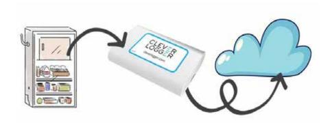
Clever Loggers are connected directly to the internet via a Gateway.
