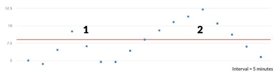
Example: The delay is set to 15 minutes. The first spike (1) does not trigger the alarm because it last less than 15 minutes. The second spike (2) triggers an alarm because the temperature remains above the threshold for more than 15 minutes.
