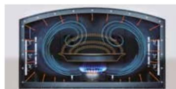
Combining a circular burner with an enamelled cast iron disk means that one single oven can cook in
