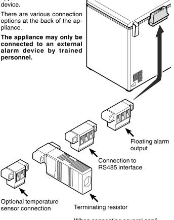
When connecting several appliances via the RS485 interface, the terminating resistor must remain on the last appliance.
