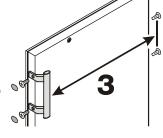
4. Transfer pin on hinge bracket to the opposite side.
