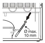
1. Drill marked section on the back of the appliance.
