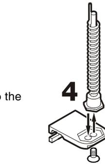
4. Transfer pin on hinge bracket to the opposite side.
