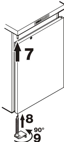
8. Insert hinge bracket in lower door mounting.
