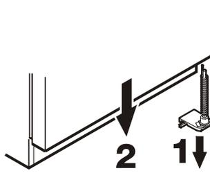
2. Pull the door out at the bottom and lift off.
