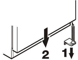
2. Pull the door out at the bottom and lift off.
