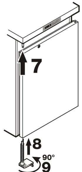
8. Insert hinge bracket in lower door mounting and screw into place.
