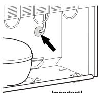
Important! 4. Close the sensor cable opening at the back of the appliance with the sealant provided.
