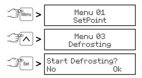
Press button  $\bigcirc$  to start defrosting or press the  $\bigcirc$  button to cancel the procedure.
