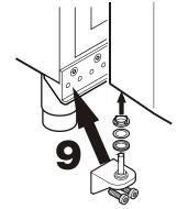
**9.** Insert hinge bracket in lower door mounting and screw to base mounting bracket.
