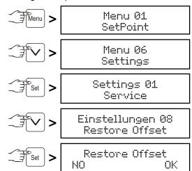
Press button to set the temperature correction values for CAL1, CAL2 and CAL3, respectively, to 0 or cancel the procedure without any changes by pressing the set button.
