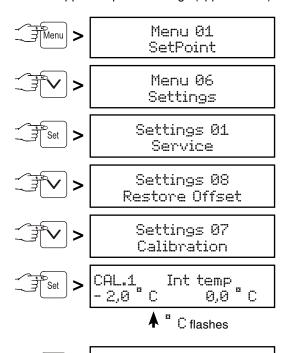
The temperature range display flashes and can be changed using the buttons  $\checkmark$  or  $\land$  (e.g. -1°C).
