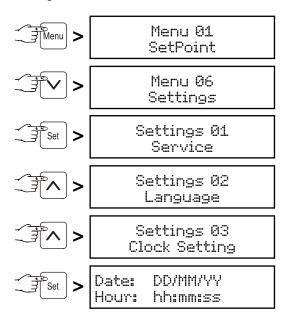
The value to be changed flashes and can be changed by pressing the buttons  $\bigvee$  and  $\bigwedge$ .
