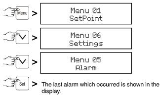
30 alarm events are saved. The highest figure (A  $\_$  ) is the last alarm which occurred. Select a previous alarm event by pressing the buttons  $\boxed{\checkmark}$  and  $\boxed{\land}$ .
