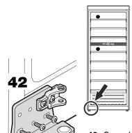
42. Screw hinge bracket into place.
