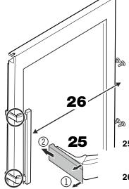
**25.** Release pressure plates at the front ① and pull them backwards to remove ②.
