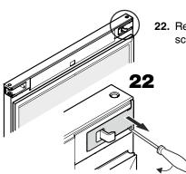
**22.** Release cover with a small screwdriver and remove.
