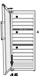
**45.** Place door on pin and move the top of it to the hinge bracket.
