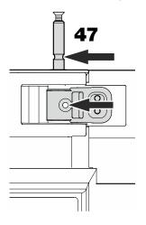
**47.** Push in hinge pin until groove in the pin lines up with bore hole in the hinge bracket.
