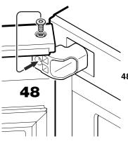
**48.** Undo screw in hinge pin and screw into bore hole in hinge bracket.
