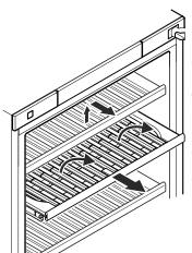
The wooden shelf above it must be removed so that the presentation shelf can be used. Raise and remove the shelf.
