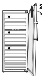
**21.** Tilt door slightly to the side and remove by lifting upwards.
